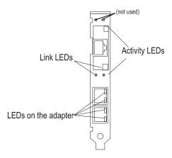
Figure 1-3. NC7132 Gigabit over copper upgrade module and LED indicators
